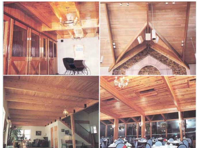
FIG 11.2 THE USE OF GLUED-LAMINATED BEAMS (RIGIDPLY RAFTERS)
