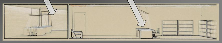
50fc on the work surfaces 20fc on the walls
