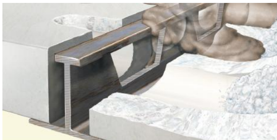
Figures 9a & 9b: Girder-Slab details. Taken from www.girder-slab.com
