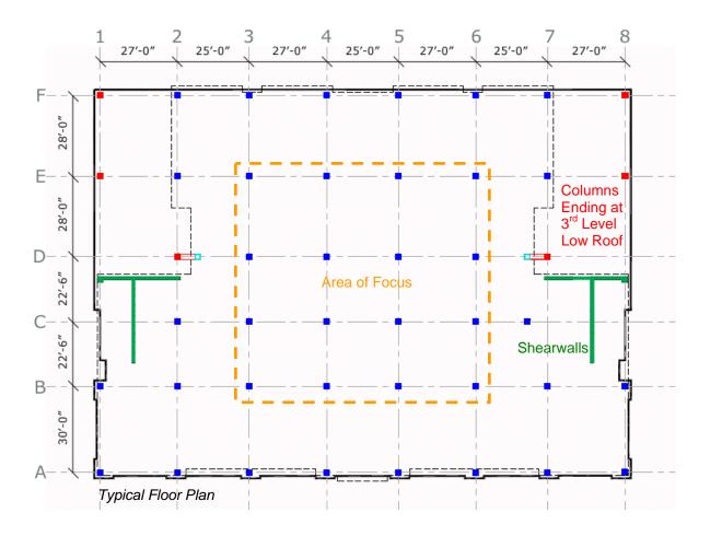
Because this building houses high-tech laboratories, vibration criteria are very important when considering alternative structural framing systems. Other considerations include cost, weight, and overall depth of the floor system.
