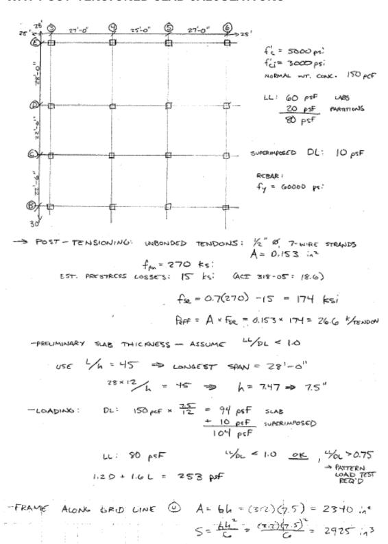
POST-TENSIONED TWO-WAY SLAB (CONT.)
