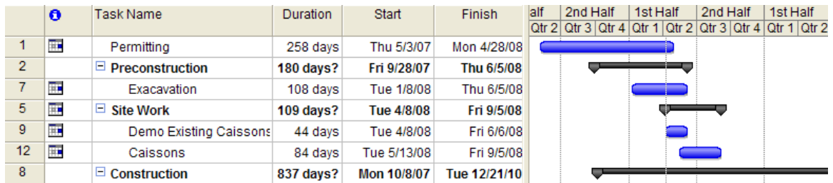
Figure 3.2 Schedule- Drilled Shaft Foundation
