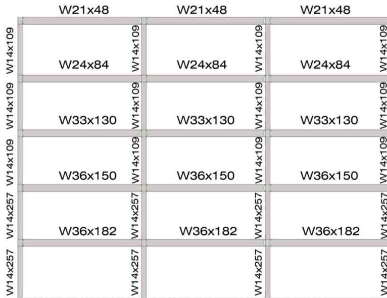
FIGURE 16 – Progressive Collapse Design
