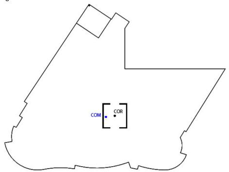
Figure 17: Shearwalls Only COM vs. COR Levels 2-4
