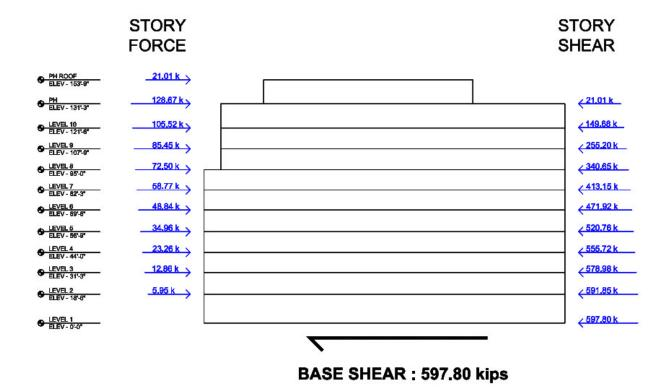
Figure 13: Seismic Force Diagram
