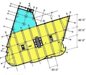
Figure 7: Slab Type Layout
