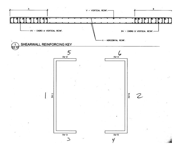
Figure 18: Shear Wall Reinforcement Layout
