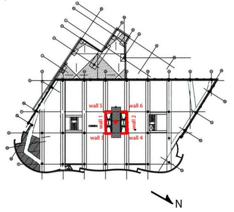
Figure 16: Lateral System (shear walls) with Labels
