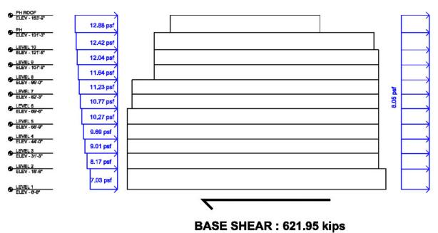
Figure 12: E/W Wind Load Diagram
