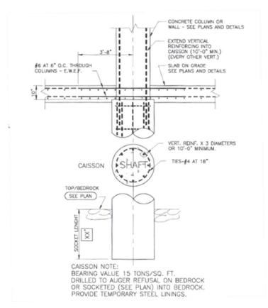
designed for a typical column reaction of 3500 kips. Brayman Construction
