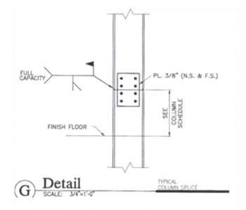
Figure 8- Splice Detail
