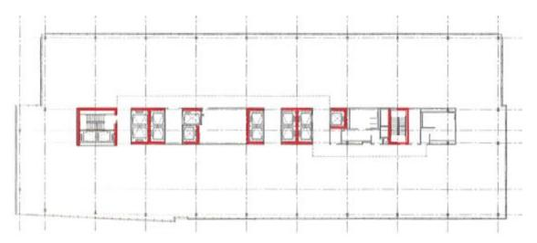
Figure 9- Shear Wall Layout
