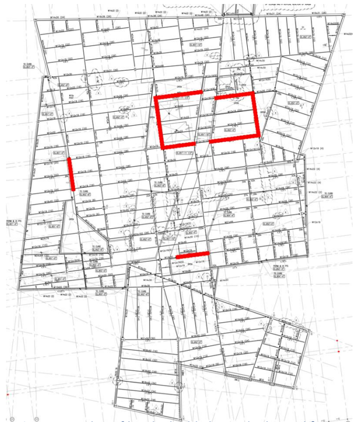
Figure 12 - Plan of level 6 highlighting the braced frames
