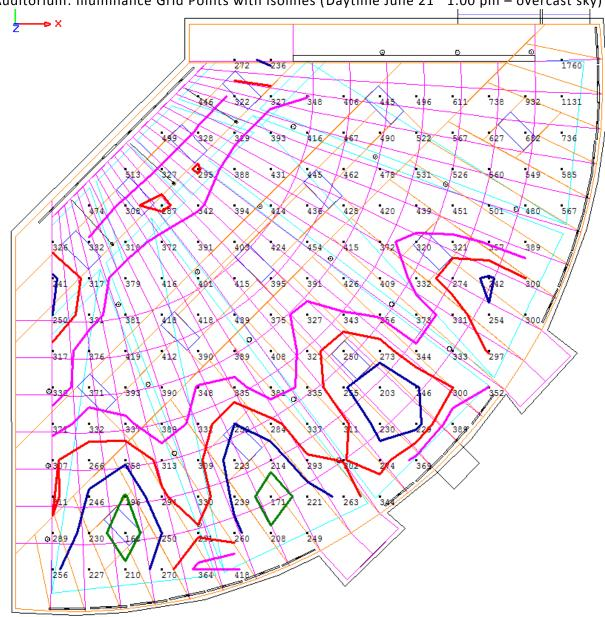
Figure 1.1 Auditorium: Illuminance Grid Points with Isolines (Daytime June 21<sup>st</sup> 1:00 pm – overcast sky)
