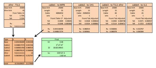
So the final  $I_{sc}$  for this circuit that ends with panelboard 1L1 comes to 1,598 Amps of fault-current.
