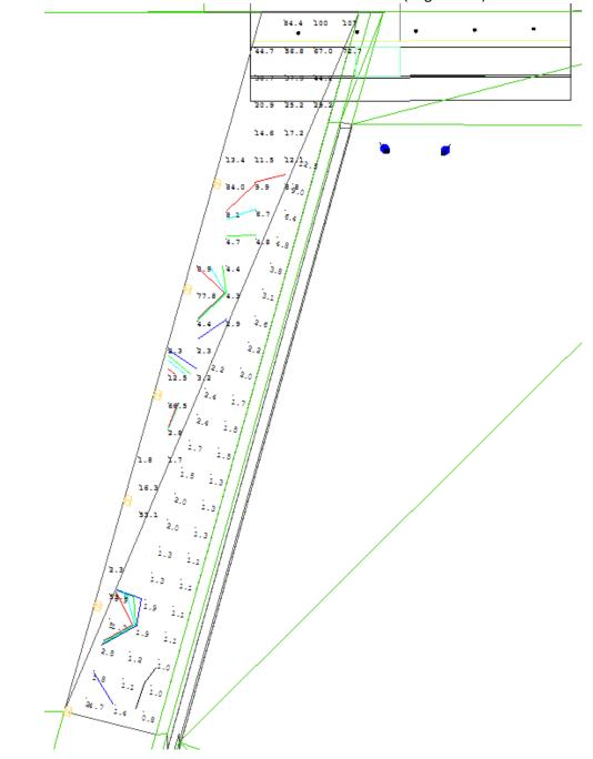
Figure 1.1 Exterior and Grounds: Illuminance Grid Points with Isolines (Nighttime)
