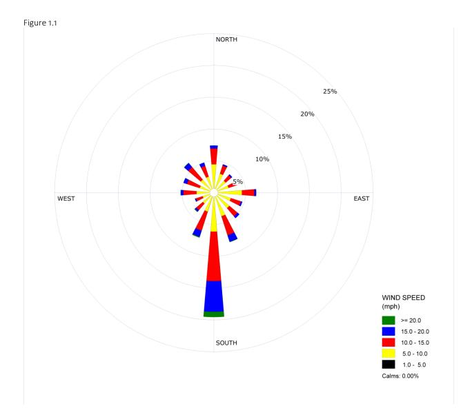
This wind rose shows that wind is mostly from the south. In order for the disks to spin, there needs to be east or west direction wind. By this wind rose, you can see that wind comes from the East 22% of the time, and from the West, also about 22% of the time. So totally, the solar disks should be able to be spinning about 44% of the day. This means they could spin up to 10.5 hours out of the day. The wind rose also shows that the average wind speed is about 10 mph.
