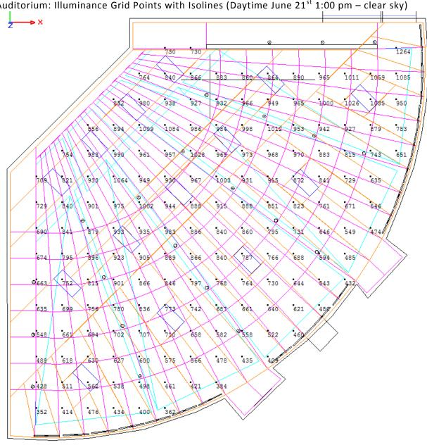
Figure 1.1 Auditorium: Illuminance Grid Points with Isolines (Daytime June 21<sup>st</sup> 1:00 pm – clear sky)
