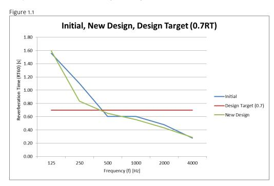
From the graph above, you can see that the  $RT_{500}$  of the new ceiling design is right underneath the target RT of 0.7. At 500 Hz the new design results in an RT of 0.65. The initial design does provide an RT of 0.6, which is also very good for this space.
