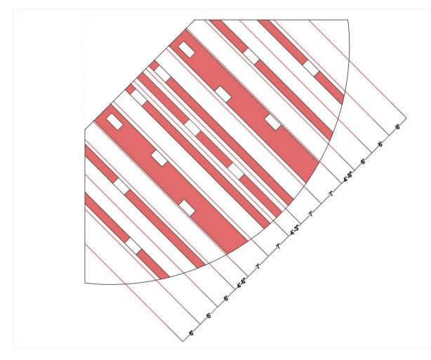
In the figure above, the skylight spans are highlighted in red to show where the structural joist <u>cannot</u> be placed. Only in the white parts could the joists span the whole length of the auditorium. Slight adjustments were needed to the placement of the skylights in order to accommodate the spans between joists. A span of 7' was chosen to be the largest span acceptable. This decision was based on the upper limitations of LH joists with they're depth and self-weight restrictions.
