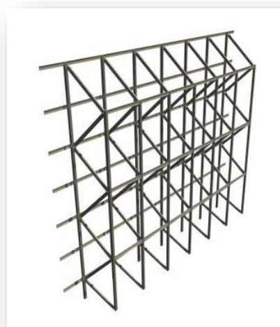
Figure 3-2: Façade Retaining Structure
