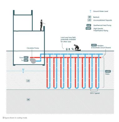
Figure 6: Vertical Well Ground Coupled Heat Pump
