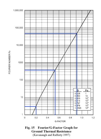
Figure A.3: Fourier/G-Factor Graph for Ground Thermal Resistance
