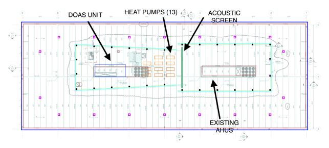
The first major change to the roof load was the removal of AHU #2 and the acoustical screen on the east side of the building. The removal of these components required the reanalysis of the supportive beams and joists; see Figures E.2 and E.3 for the structural calculations. This analysis
