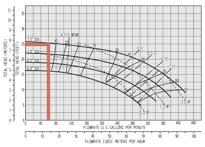
Figure C.2: Pump Selection for Hot/Chilled Water Loops
