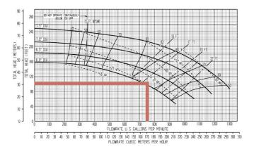
Figure 9: Pioneer SC54C75 Pump Curve
