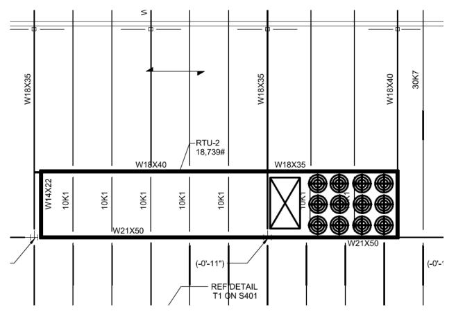
Typical Joist Design for 6 - @ 3 Tributory Area Ø 0 Un Factored Louds Dead Roof Deck Joist Ceiling 44 6 Live 30 pst 40 psf Factored Loads 1.2 (OL) +1,6 (LA) = 1.2(10psf) +1.6(30psf)=60psf Wu= 60 pst . 5' = 300 ## PLF Using LRFD 28K7 → 367plf, 152plf 300 ptf + 12(11.8) = 314.16 < 367 ptf WTL = (10psf +30psf) 5'= 200 pH = 133.3 pH < 152pH 1.5 28k7 mechs Begurements for Load and Depth
