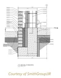
**Panel Walls |** The metal panel walls, found in the upper floors of the Engineering Center, include a zinc faced composite wall panel connected to the structure with adjustable framing angles which allows for room for an air space and XPS-1 extruded-polyestrene board insulation followed by the concrete masonry unit wall assembly.
