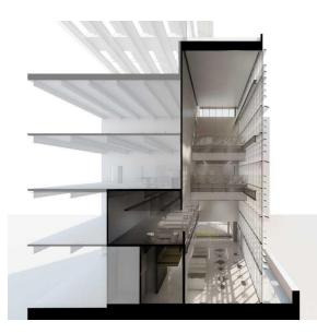
Atrium Section showing exterior glazing and shading louvers | Courtesy of SmithGroupJJR
