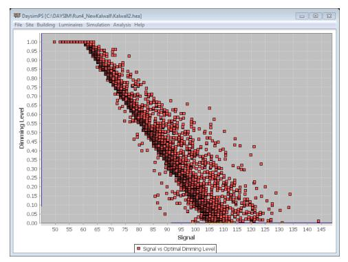
Figure 62 Signal vs. Dimming Level Plot
