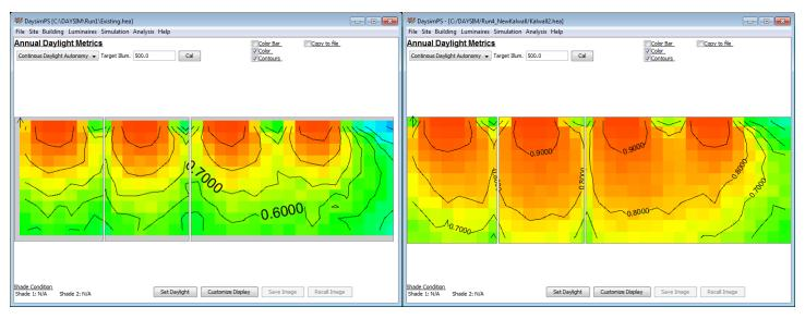
Figure 52 Continuous Daylight Autonomy Comparison
