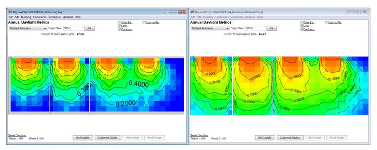
Figure 51 Daylight Autonomy Comparison (27.58 without, 66.67 with skylights)
