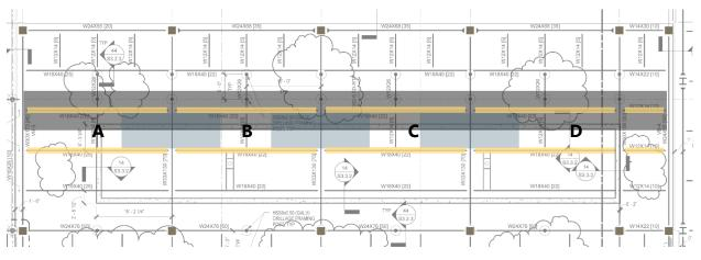
Figure 68 Altered Layout with Beam Tributary Areas Highlighted
