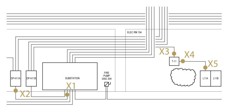
Figure 43 Enlarged One-Line Showing Fault Locations
