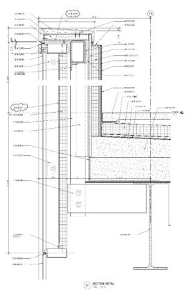
Figure 71 Roof Construction Section
