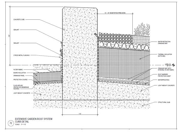
Figure 67 Green Roof Section Detail
