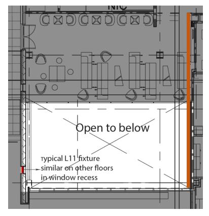
Figure 13 Level Three Atrium Lighting Plan
