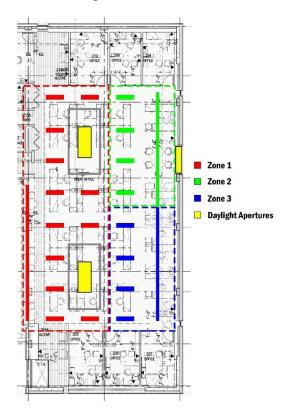
Figure 72 | Office Lighting Daylight Zones
