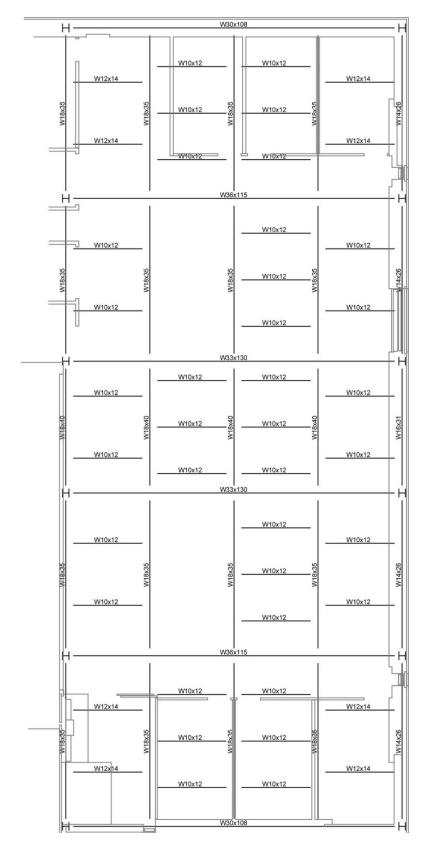
Figure 69 | Designed Steel Structural Layout
