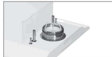
Duct installation of the exhaust valve.
