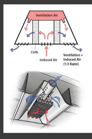
Active Chilled Beam. From Labs 21: Chilled Beams in Laboratories
