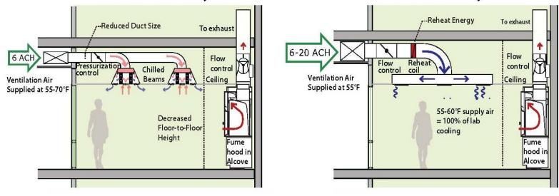
Chilled Beam vs. VAV system. From Labs 21: Chilled Beams in Laboratories
