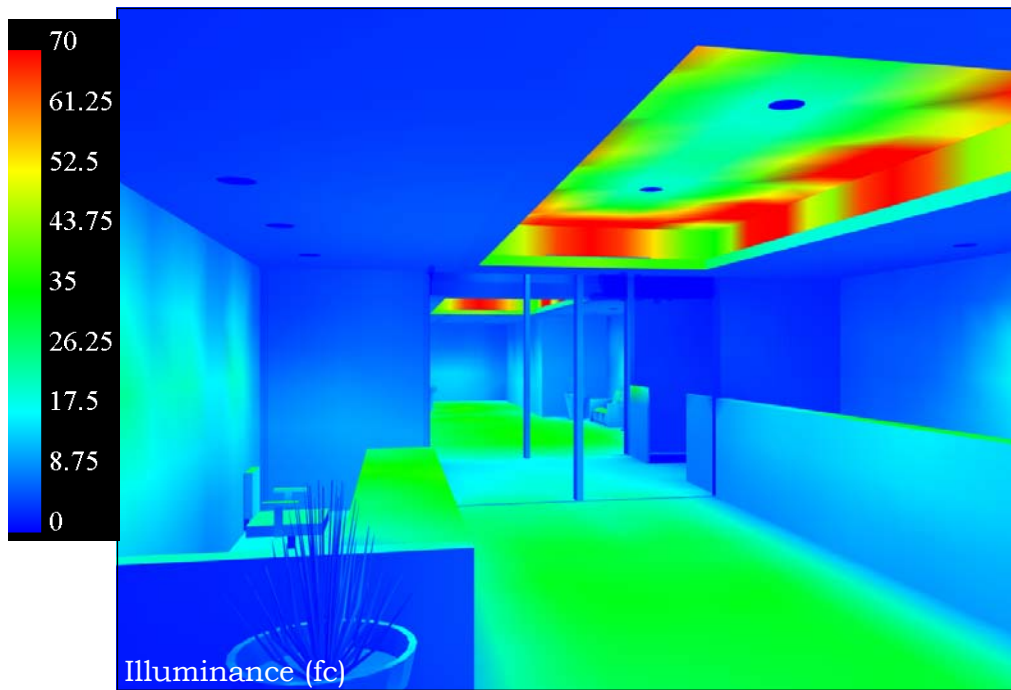
The ceiling coves, while much brighter than the surroundings, create an even distribution onto the corridor floor. The downlights illuminate the walls and workplane, and take focus away from the coves.
