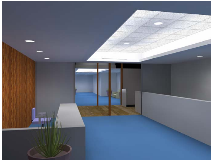
The ceiling coves, while much brighter than the surroundings, create an even distribution onto the corridor floor. The downlights illuminate the walls and workplane, and take focus away from the coves.
