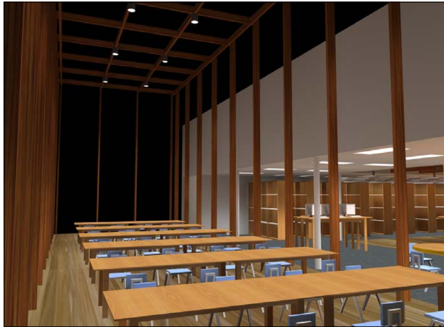
The metal-halide canister lamps provide even distribution and acceptable contrast ratios when little to no sunlight is illuminating the space.
