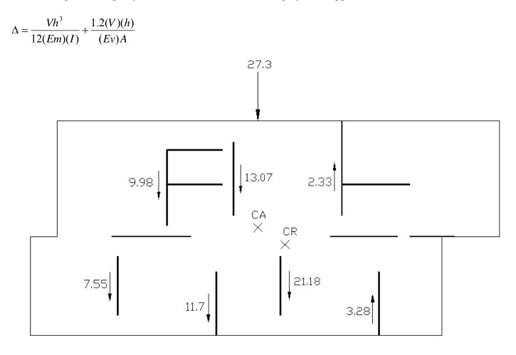
Figure 7 – Distribution of Forces onto N-S Shear Walls
