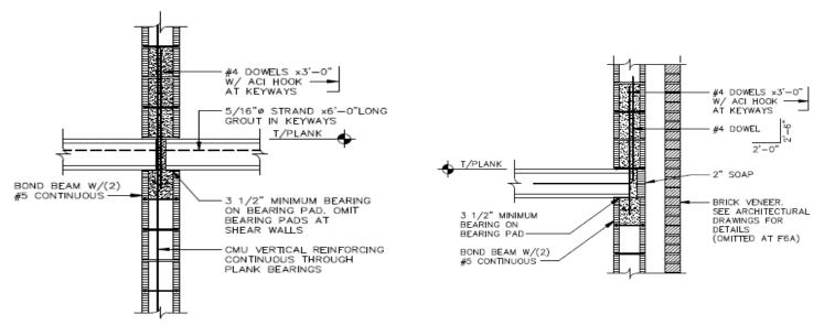
Figure 5 – Floor Planks at Interior Walls
