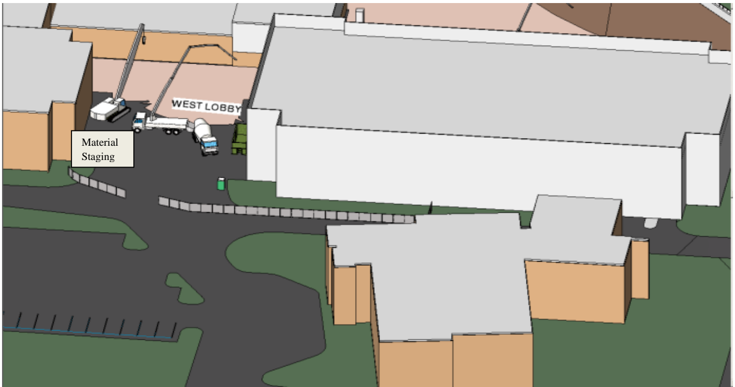
Figure 11: Site Logistics for project- West Lobby Area
