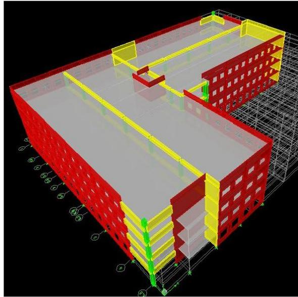
Drift calculations were determined by ETABS. The computer program calculated a maximum drift of 0.21" in the y-direction and 0.15" in the x-direction. Industry standards restrict a building to drift no more than  $H/400$ . This would allow the top story to deflect a maximum of 1.68". Clearly, drift in each direction does not control the design of the shear walls.
