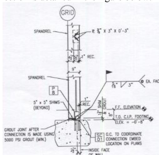
There is another connection used to secure the shear walls to the foundation. Lenton manufactures an interlocking rebar system which is utilized to resist the tensile forces caused by overturning. Details of this system are shown below.
