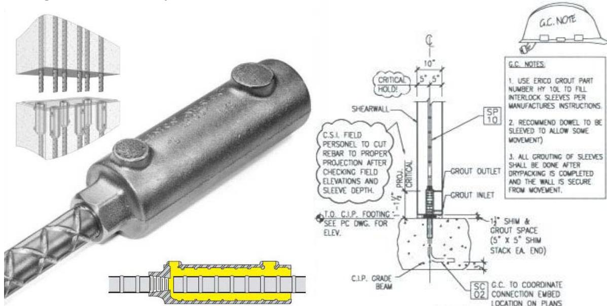
When the panels arrive on site, they are placed over dowels protruding out of the foundation. The Lenton connectors slide over the dowels and is then pumped with grout. When the grout cures, the connection provides a continuous link from the top shear wall to foundation. This detail is also used when connecting panel to panel.
