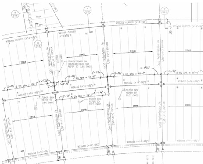
Figure 1c. Curved 3-Story Floor Framing 1
