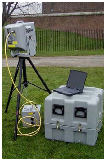
Figure 5 Laser Scanning Equipment (CyraX 2500)
