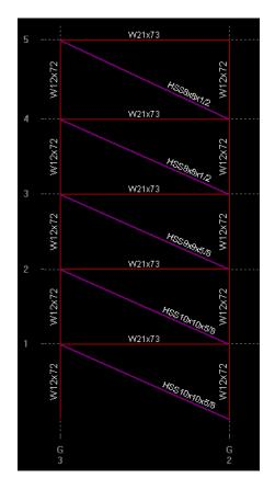
Figure 9: Braced Frame 3
