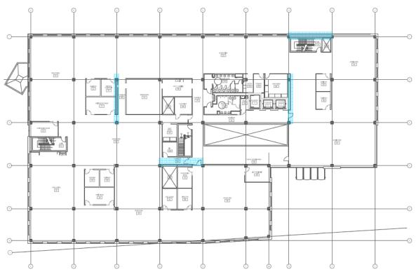
Figure 27: Original Second Floor Plan and Location of Braced Frames
