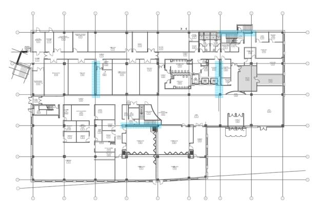
Figure 25: Original First Floor Plan and Location of Braced Frames
