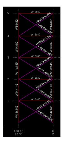
Figure 18: Braced Frame 3
