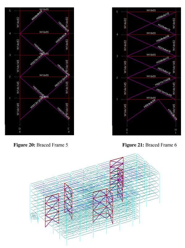
Figure 22: 3-D Layout of Structural System
