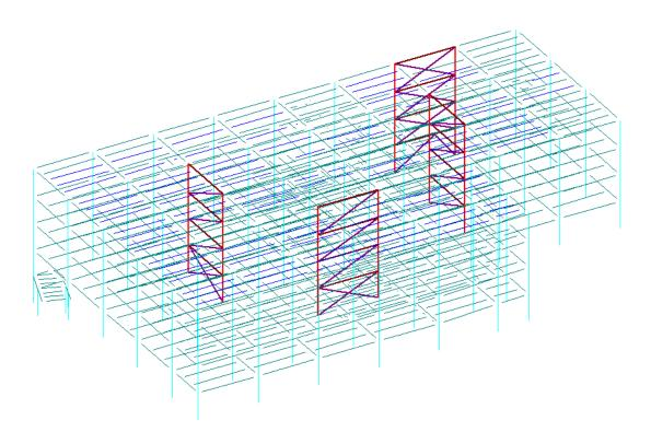
Figure 6: 3-D Layout of Structural System
