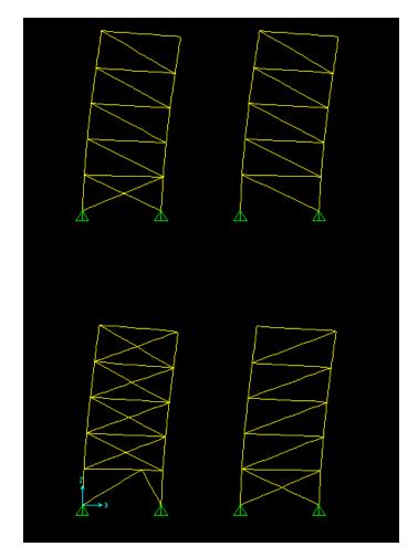
Figure 13: Deflected Shape of Braced Frames in SAP 2000
