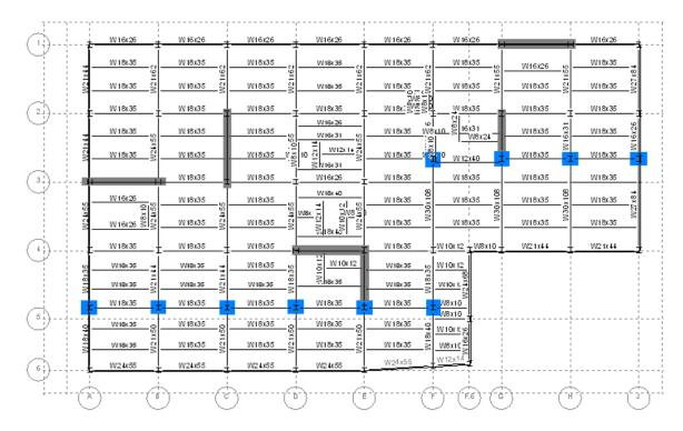
Figure 15: Revised Column and Braced Frame Layout
