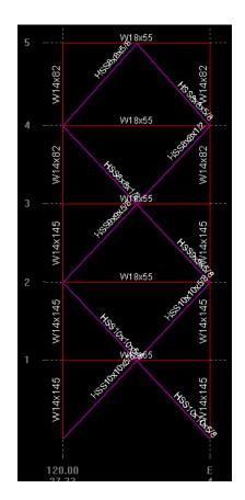
Figure 17: Braced Frame 2
