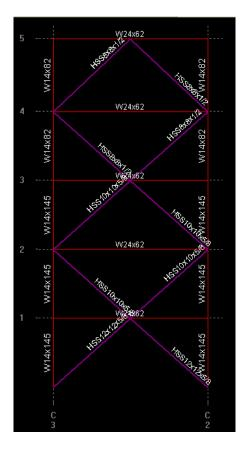
Figure 16: Braced Frame 1
