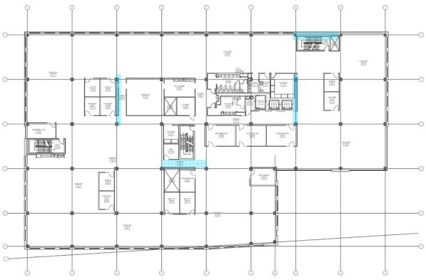
Figure 29: Remaining Original Floor Plans and Location of Braced Frames
