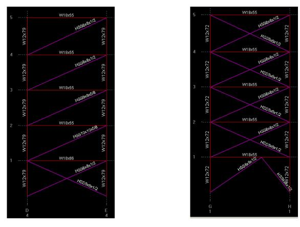
Figure 10: Braced Frame 2
