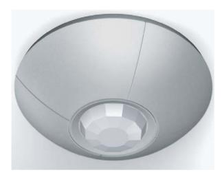
The LOS-CIR Series ceiling-mount passive infrared sensors can integrate into Lutron systems or function as standalone controls using a Lutron power pack. The sensor uses a small semiconductor heat detector that resides behind a multi-zone optical lens. The sensor's detector is sensitive to the heat emitted by the human body. In order to trigger the sensor, the source of heat must move from one range of detection to another. Non-moving hot objects will not cause the lights to turn on.
