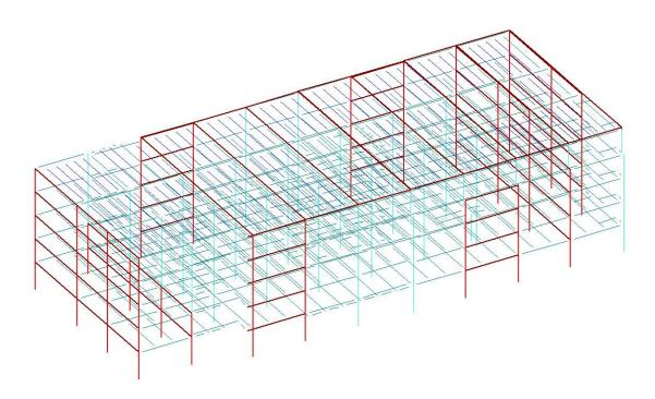
FIGURE 3 – Overall 3D RAM Model with highlighted moment frames
