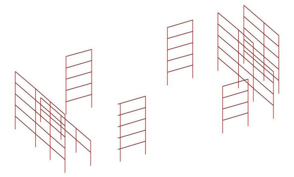
FIGURE 4 - 3D RAM Model with only moment frames
