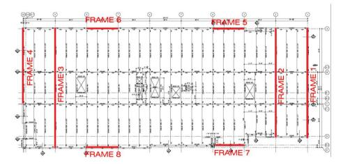
FIGURE 2 – Typical Floor plan with moment frames
