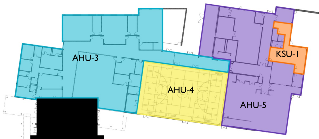
Figure 2: Wing B AHU Distribution
