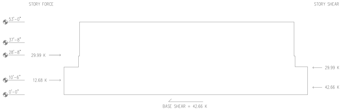
Figure 30 – “Building 2” Seismic Loads
