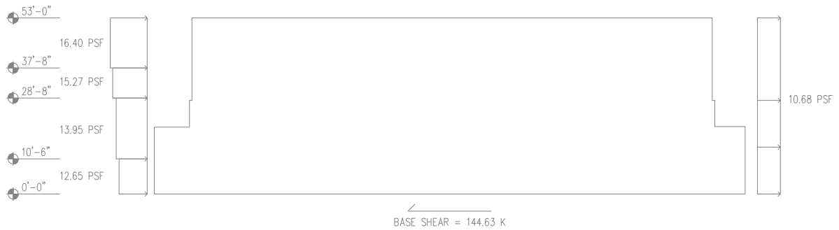
Figure 26 – “Building 1” Wind Loads (North/South)
