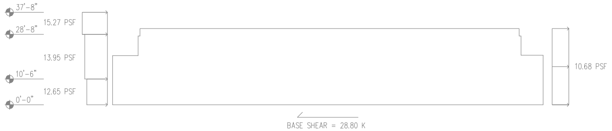
Figure 27 – “Building 4” Wind Loads (North/South)
