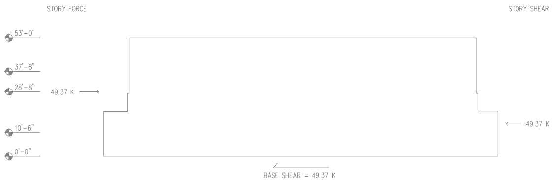
Figure 32 – “Building 4” Seismic Loads
