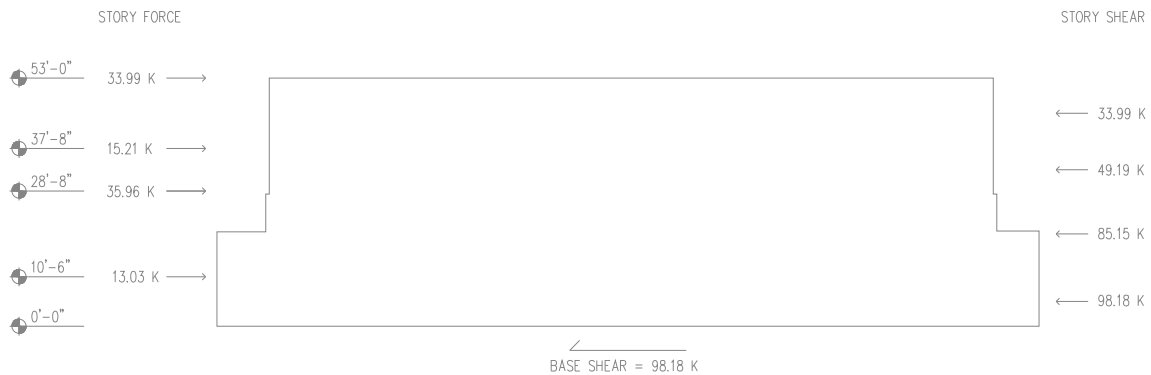
Figure 29 – “Building 1” Seismic Loads
