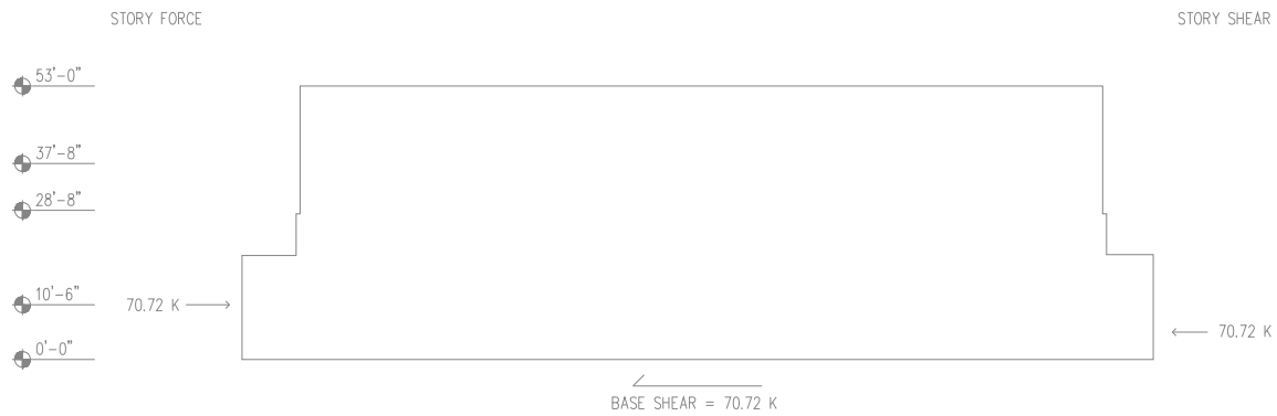
Figure 31 – “Building 3” Seismic Loads
