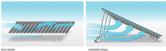
flow through the panels allowing them to be installed without roof penetration, attachments, or ballasts, making installation quicker, easier, and cheaper than conventional models. This also makes the panels easily removable for roof maintenance.
