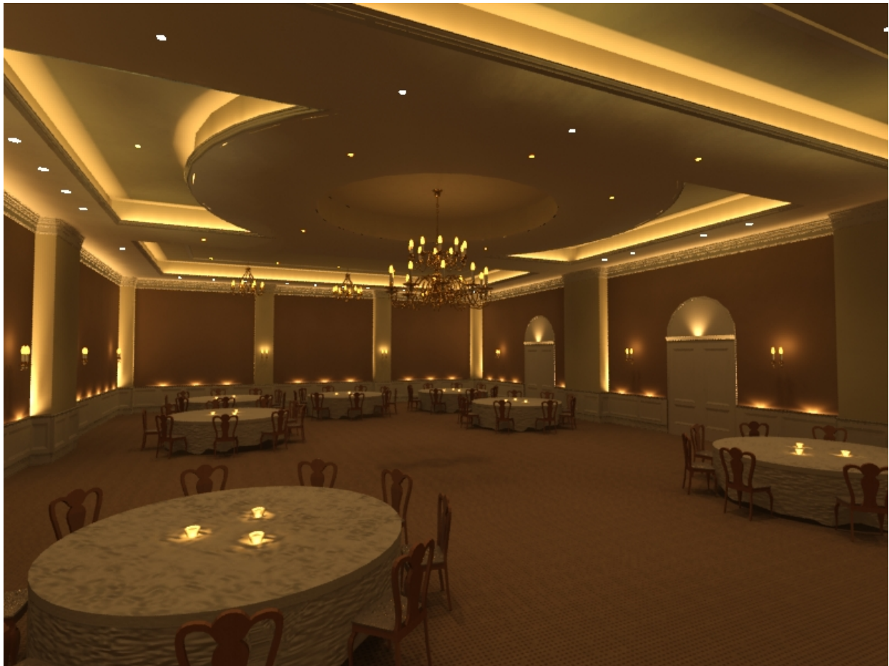
Figure 65: Ballroom dining setting – downlights dimmed to 10%, sconces switched on, perimeter glow switched on.
