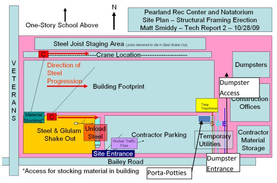
Figure 4-4.3 – Structural Framing Erection Phase Site Plan
