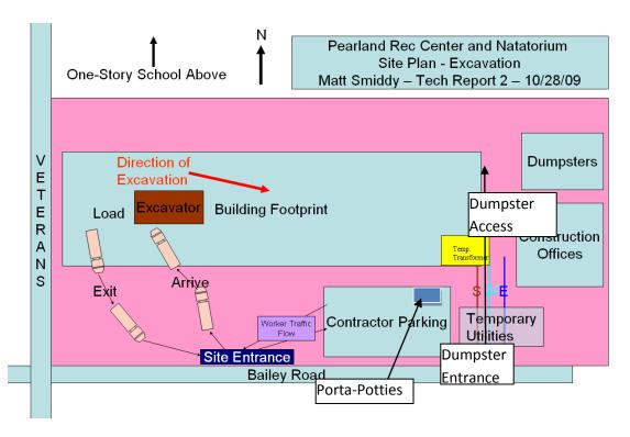
Figure 4-4.1 – Excavation Phase Site Plan
