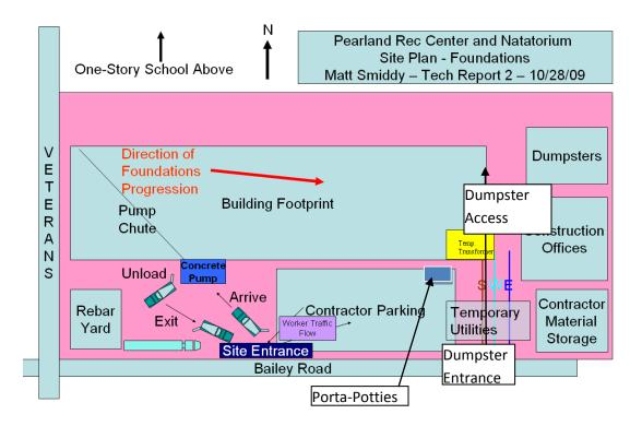
Figure 4-4.2 – Foundations Phase Site Plan
