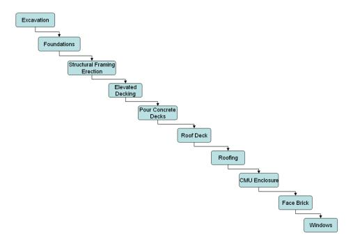
Figure 5-2.2 – Structural and Enclosure Trade Construction Sequence
