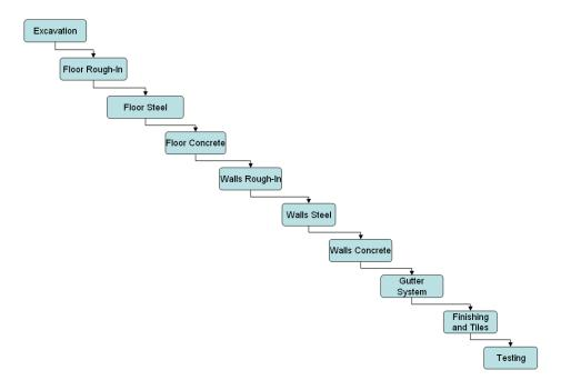
Figure 5-2.5 – Swimming Pool Construction Sequence
