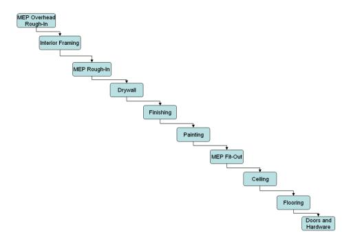
Figure 5-2.3 - Interior Trades Construction Sequence
