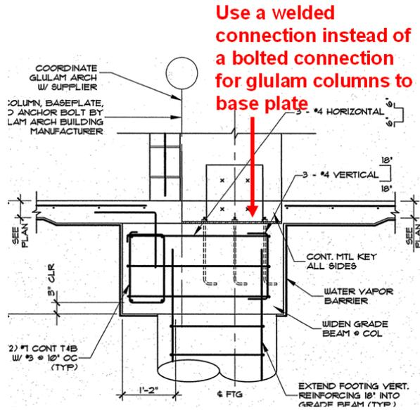
Figure 2-5: Glulam Column Connection Detail
