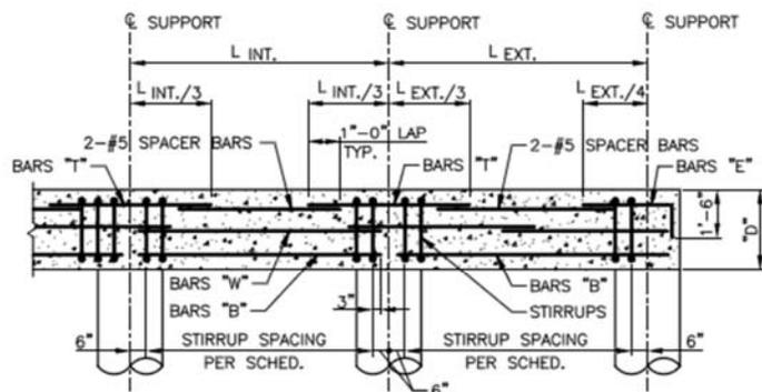
Typical Grade Beam Reinforcing Detail
