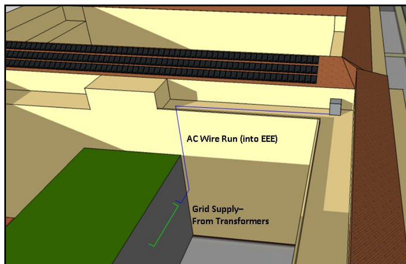
Figure 38: AC Wire Run from Inverter to Grid Connection/Distribution Panel in EEE
