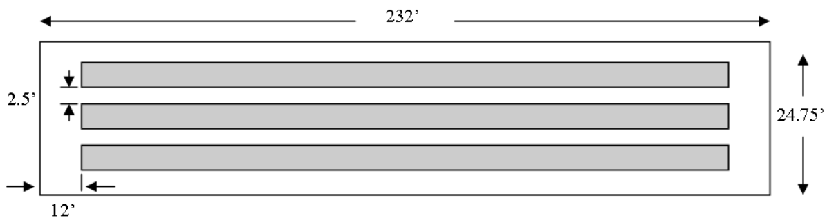
Figure 31: PV Panel Layout, each row contains 64 individual panels
