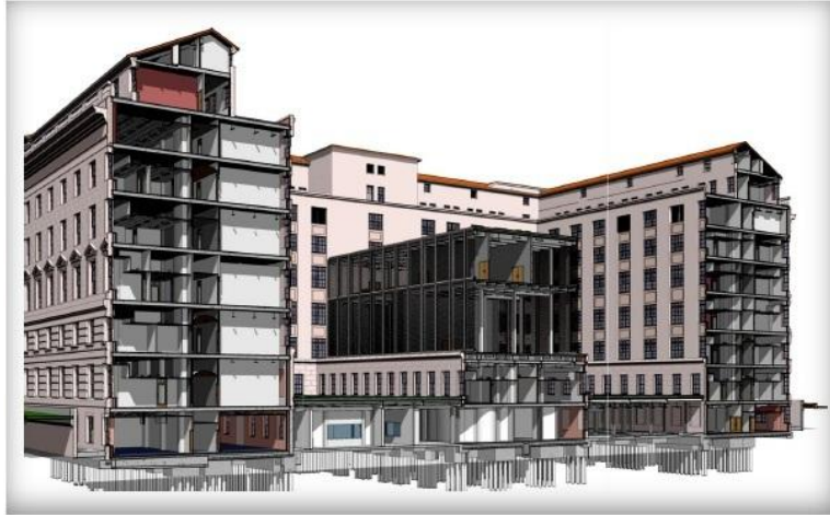
Figure 3: Section through Courtyard 1 of the Office Renovation Building showing the structure's new EEE
