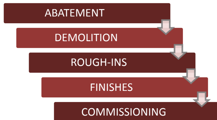
Figure 9: Floor by floor critical path schedule for interior renovation work
