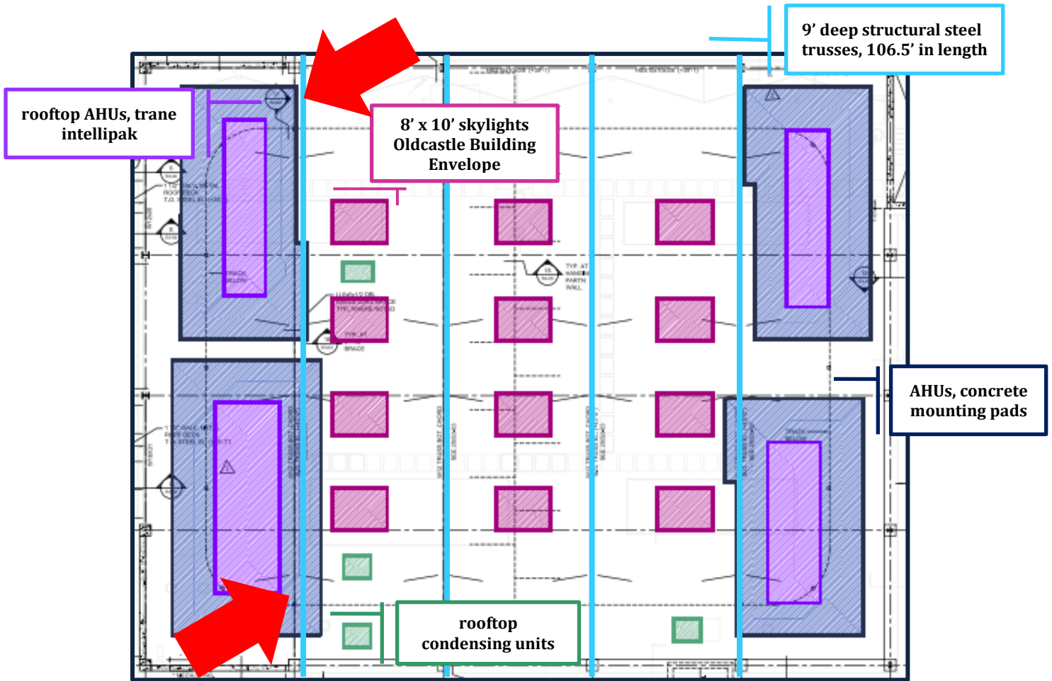
figure s.2 -Updated Roof Mechanical Equipment Plan
