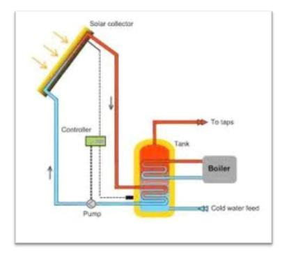
Figure 3 - Solar Thermal Storage System
