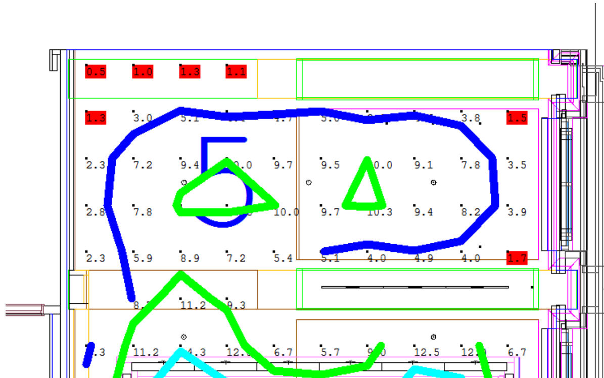
Figure 15: Lounge Entrance | Illuminance values highlighted below 2.0 fc
