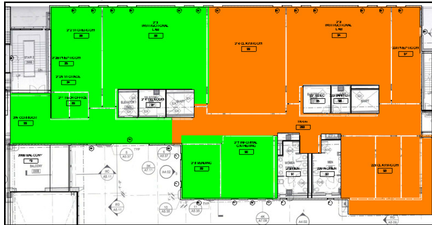
Fig.3: Lab and non-lab spaces on same AHU's
