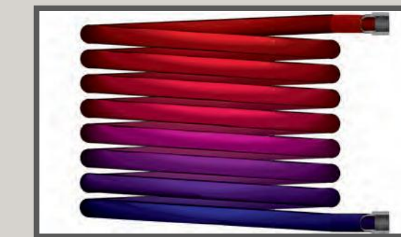
Plain tube internal heat exchangers required on the solar and load side
