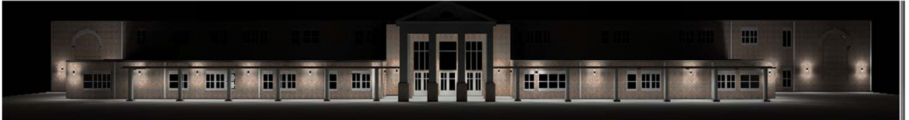
Figure 6: Covered Entrance and Covered Walkways with Type A1 ,B1, C1 Luminaires on
