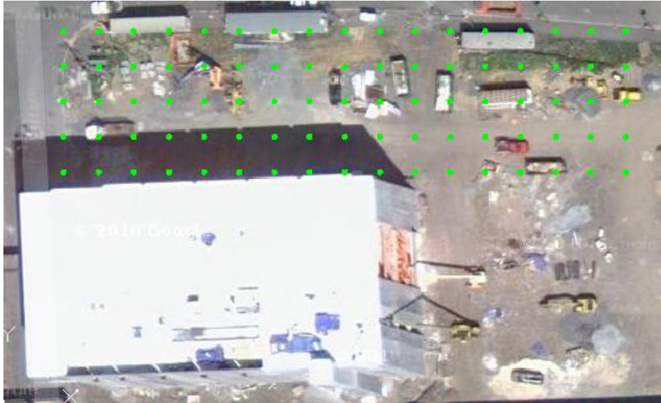
Figure 5-Schematic of bore hole positions with proper spacing
