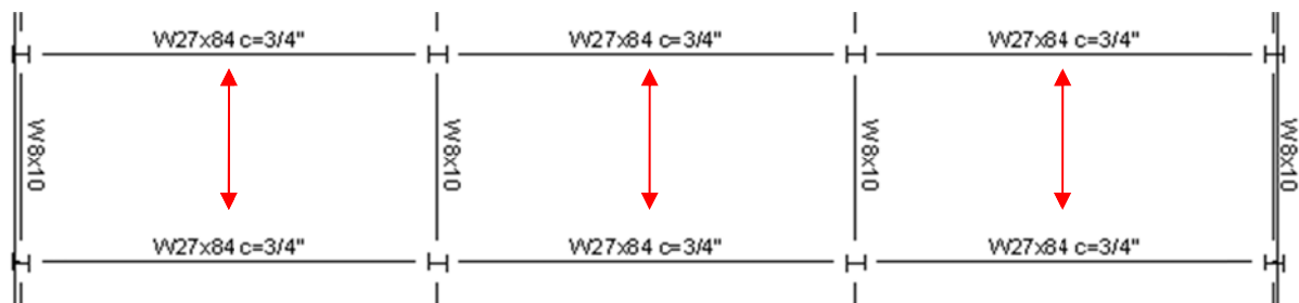
Figure 16: Ram Structural System Precast Plank Steel Beam Design
