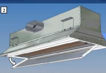
wer the front edge of the return air panel when the edge of e panel clears the grille extrusion
