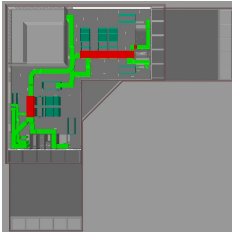
Figure 69: Laboratory Supply System on Penthouse Level. Manifolds are shown in Red, while the Supply Mains are Green and the Air Handlers are Teal.
