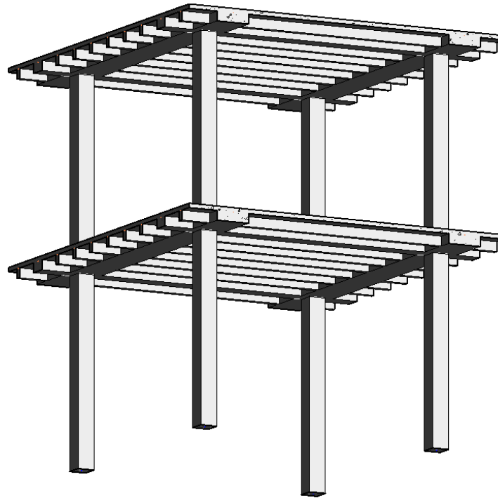
Figure 62: 3D View: Redesigned Pan-Joist System Typical Bay.
