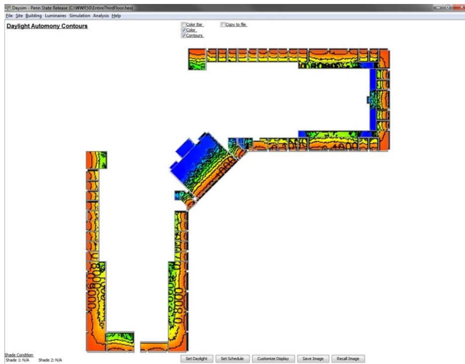
WWR 50 Third Floor DA 322.8 lux
