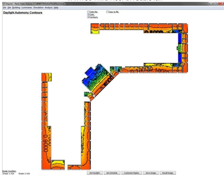
WWR 70 Third Floor DA 322.8 lux
