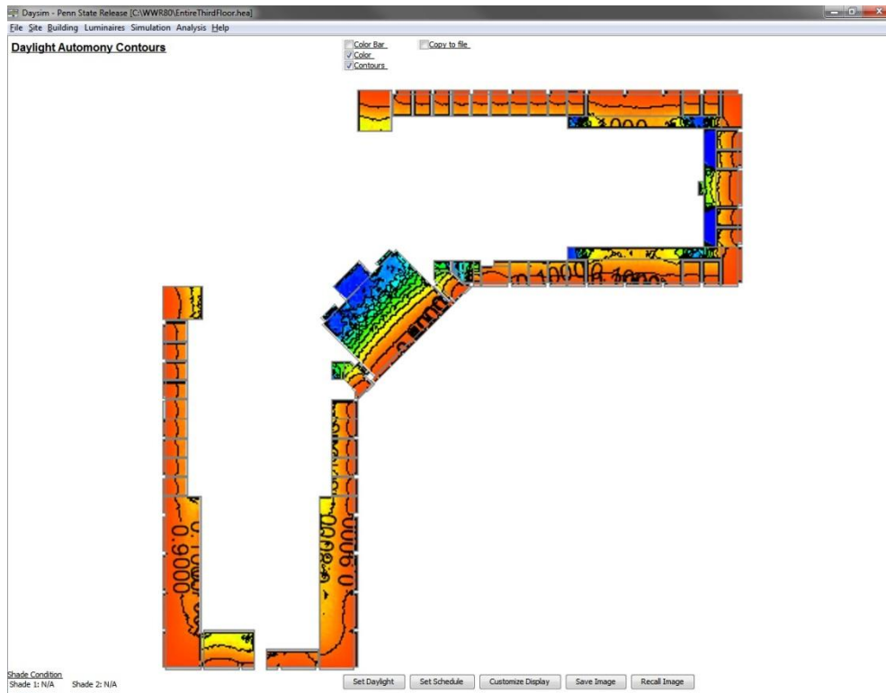
WWR 80 Third Floor DA 322.8 lux
