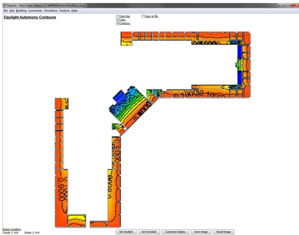
WWR 90 Third Floor DA 322.8 Lux
