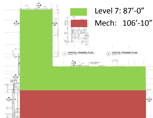
Figure 8- Showing the different roof levels on the building
