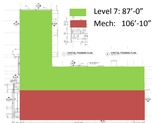
Figure 9- Showing the different roof levels on the building
