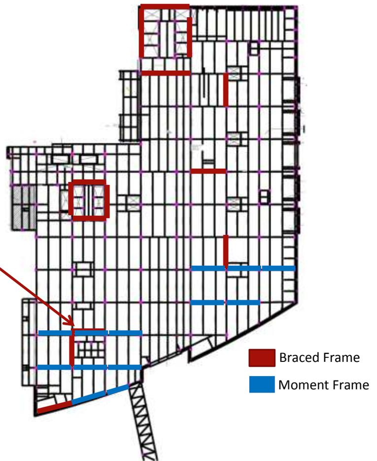
**Figure 10 - Typical Braced Frame**
