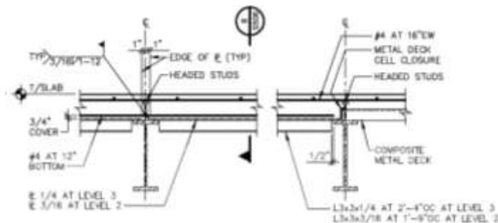
**Figure 7 – Slab Detail; Radiation Shielding Plate**
