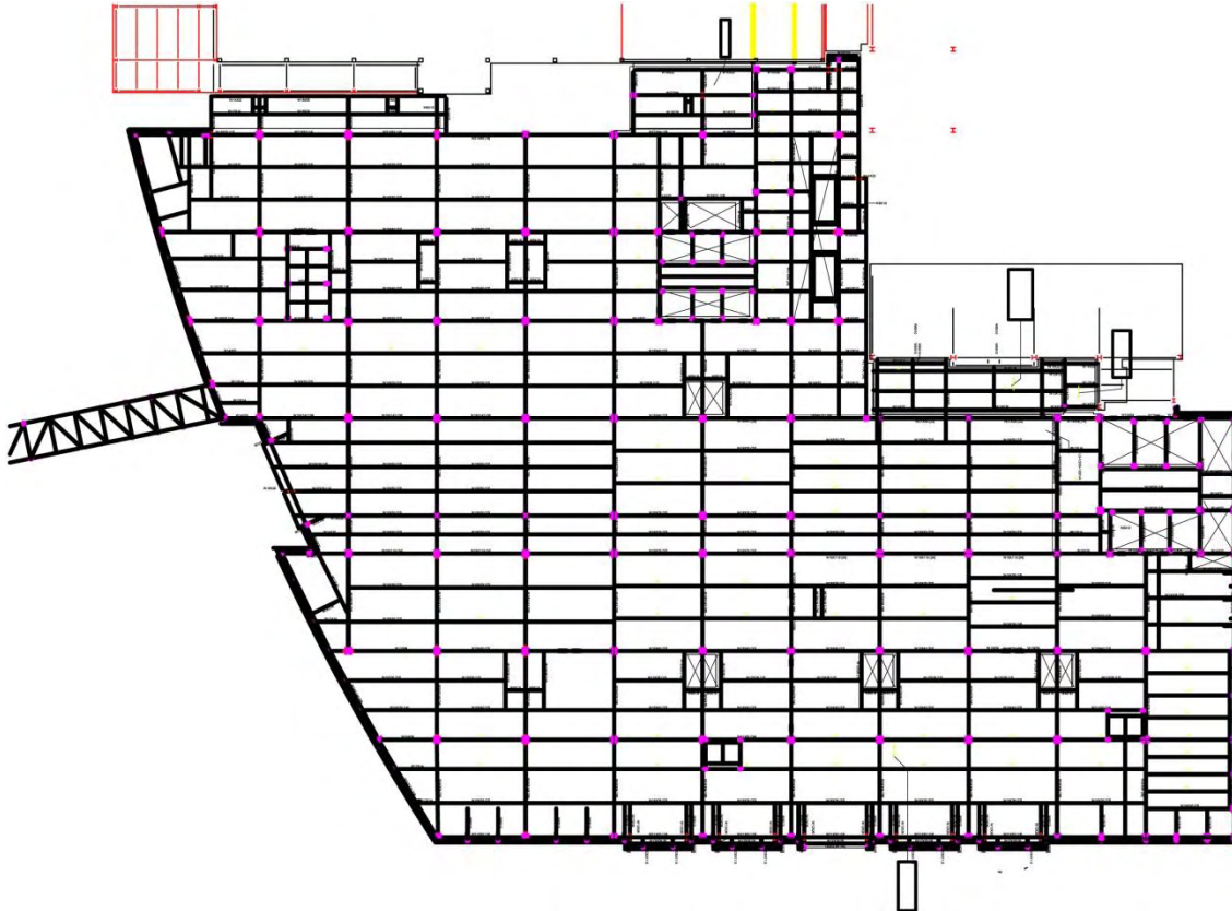
Figure 17 – Typical Column Layout
