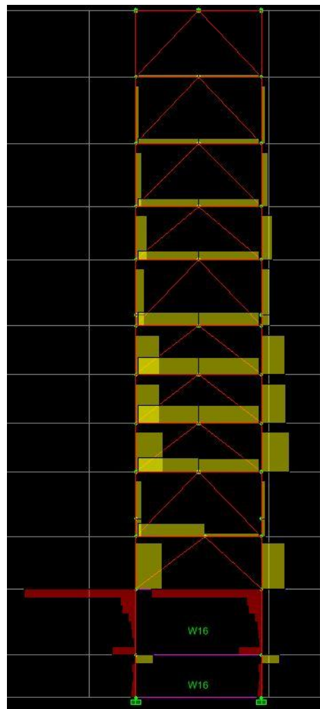
Figure 20 – Shear Reversal in Braced Frame
